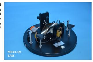
Main constructional differences between versions are in size of buckets and used funnel outflow nozzles.
